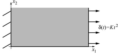
**Figure 2.** Studied brittle structure with boundary conditions.
