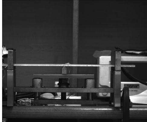
Figure 8. A photo of a three-point bending setup for beam specimens.
