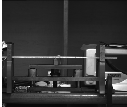
Figure 8. A photo of a three-point bending setup for beam specimens.
