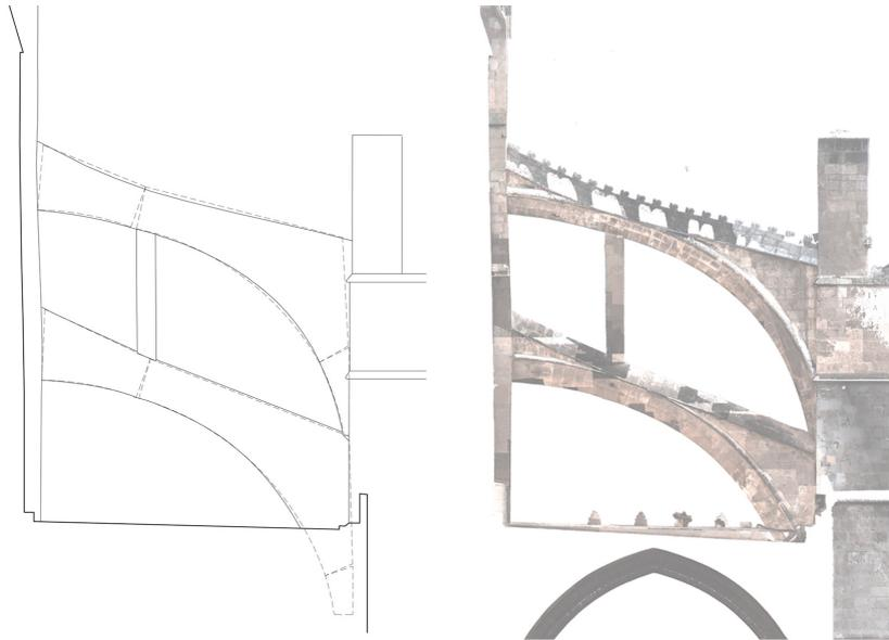
**Figure 12.** Comparison of the theoretical deformation (dashed line) with the real deformation (continuous line) (left) and orthophoto of the south flying buttresses B1 (right) (based on the point cloud by Rex Haberland).
