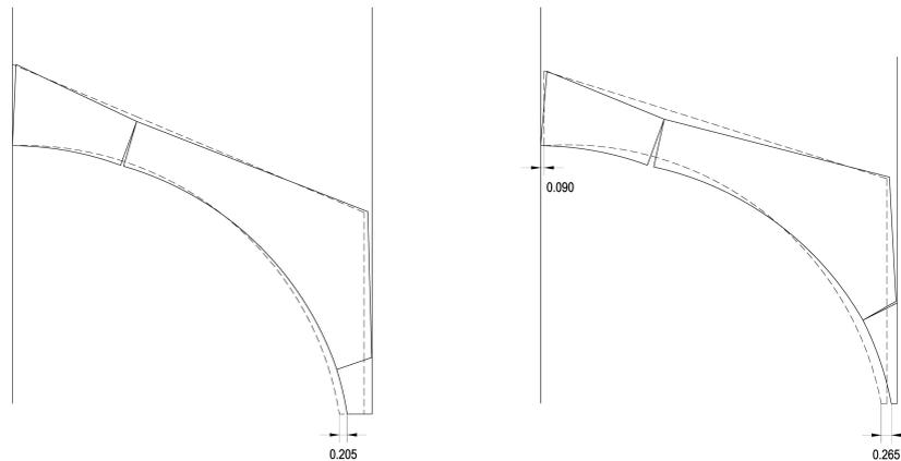
**Figure 11.** Theoretical deformation of the ideal flying buttress for the leaning of the south buttress B1 and the leaning of the nave wall. Geometry previous the deformation in dashed line: lower flying buttress (left) and upper flying buttress (right).
