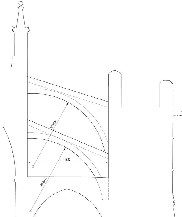
**Figure 9.** Ideal geometry considered for the structural analysis.
