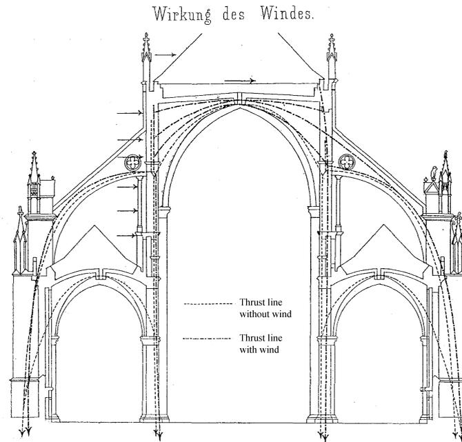
**Figure 1.** Cross section of the cathedral of Strasbourg showing the thrust line with and without wind [Ungewitter 1890]. Dotted line: thrust line without wind. Dotted-dashed line: thrust line with wind. Note that, with wind, the thrust line goes through the wall over the transverse arches.
