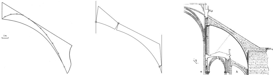
**Figure 3.** Left: passive line of thrust in the flying buttress of Nôtre-Dame, Paris [Heyman 1966]. Center: flying buttress of Nôtre-Dame with a spreading of the abutments. Right: partial cross-section of Nôtre-Dame [Viollet-le-Duc 1854].
