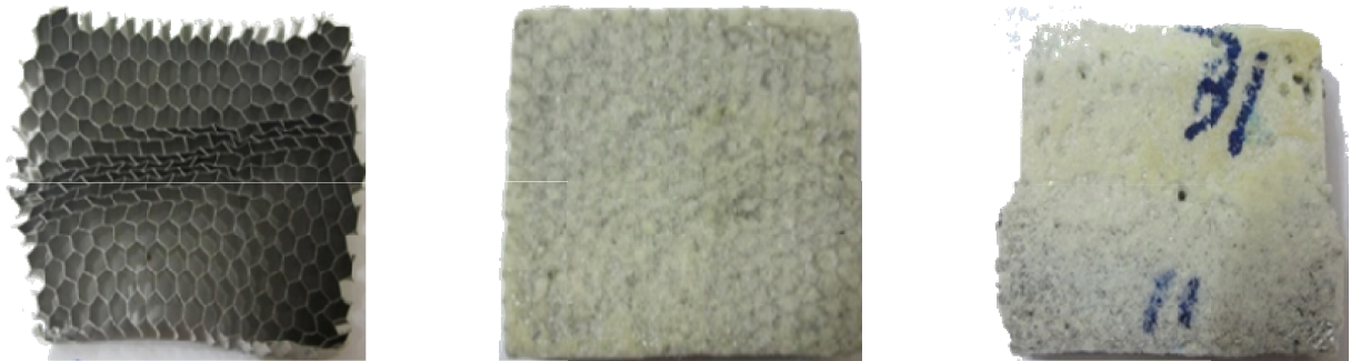
Figure 11. Final deformation modes of three structures for in-plane quasistatic tests for without foam (left), nongraded graded foam (middle) and graded foam models (right).
