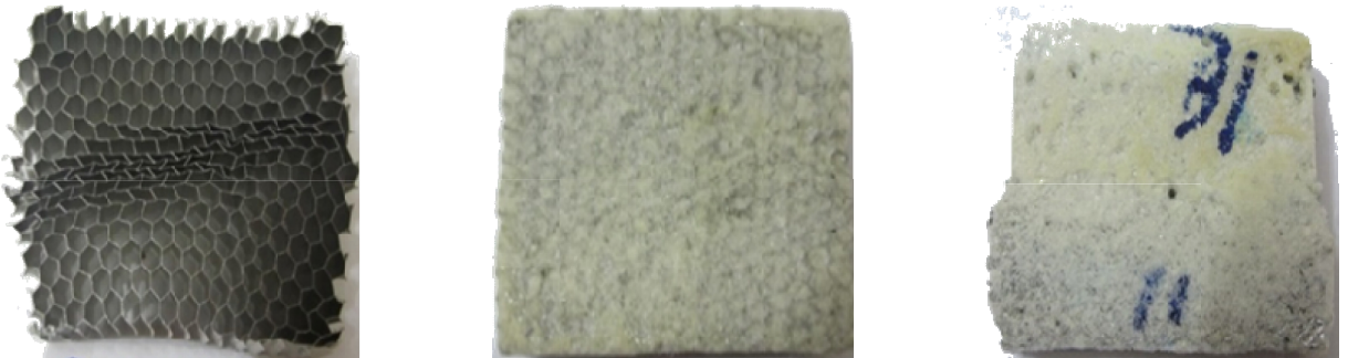
Figure 11. Final deformation modes of three structures for in-plane quasistatic tests for without foam (left), nongraded graded foam (middle) and graded foam models (right).
