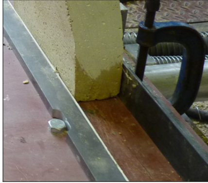
Figure 3. Support conditions for arch samples on shaking table with rubber padded metal brackets on both intrados and extrados to prevent sliding, while a degree of rotation can be expected.
