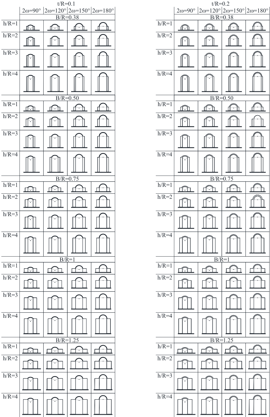
Figure 4. Geometry of analyzed buttressed arches: thin arch thickness, t/R = 0.10 (left column) and medium arch thickness, t/R = 0.20 (right column).
