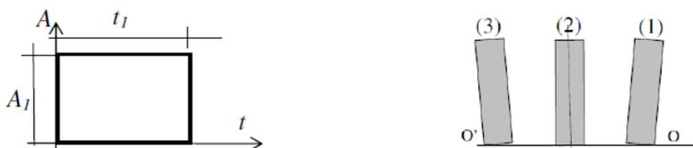
**Figure 1.** Constant horizontal acceleration impulse.
