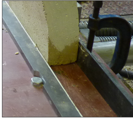
Figure 3. Support conditions for arch samples on shaking table with rubber padded metal brackets on both intrados and extrados to prevent sliding, while a degree of rotation can be expected.
