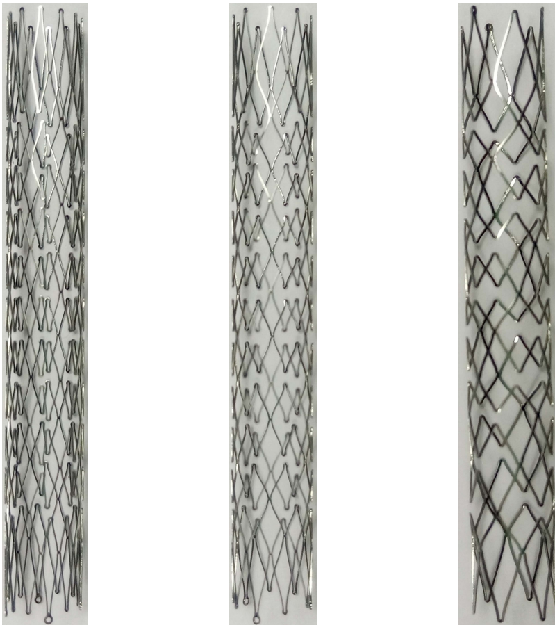
Figure 4. The three fabricated stents with varying crown numbers in the circumferential direction: 12 crown design (left), 9 crown design (middle) and 6 crown design (right).
