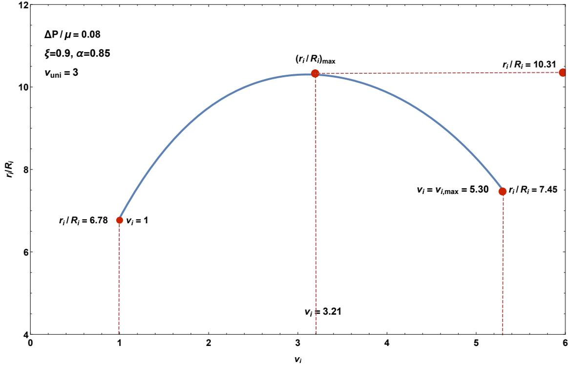
**Figure 11.** Inflation in terms of  $r_i/R_i$  as a function of  $v_i$  for (33) with  $\Delta V/R_i^3 = 3.20$ , which correspond to the sequence of inflation graphs in figures 5 and 6. This specific figure corresponds to  $\Delta P = 0.08\mu$ . The graph is well behaved, first monotonically increasing (where the correlation is with Figure 5) and then monotonically decreasing (correlated with Figure 6).
