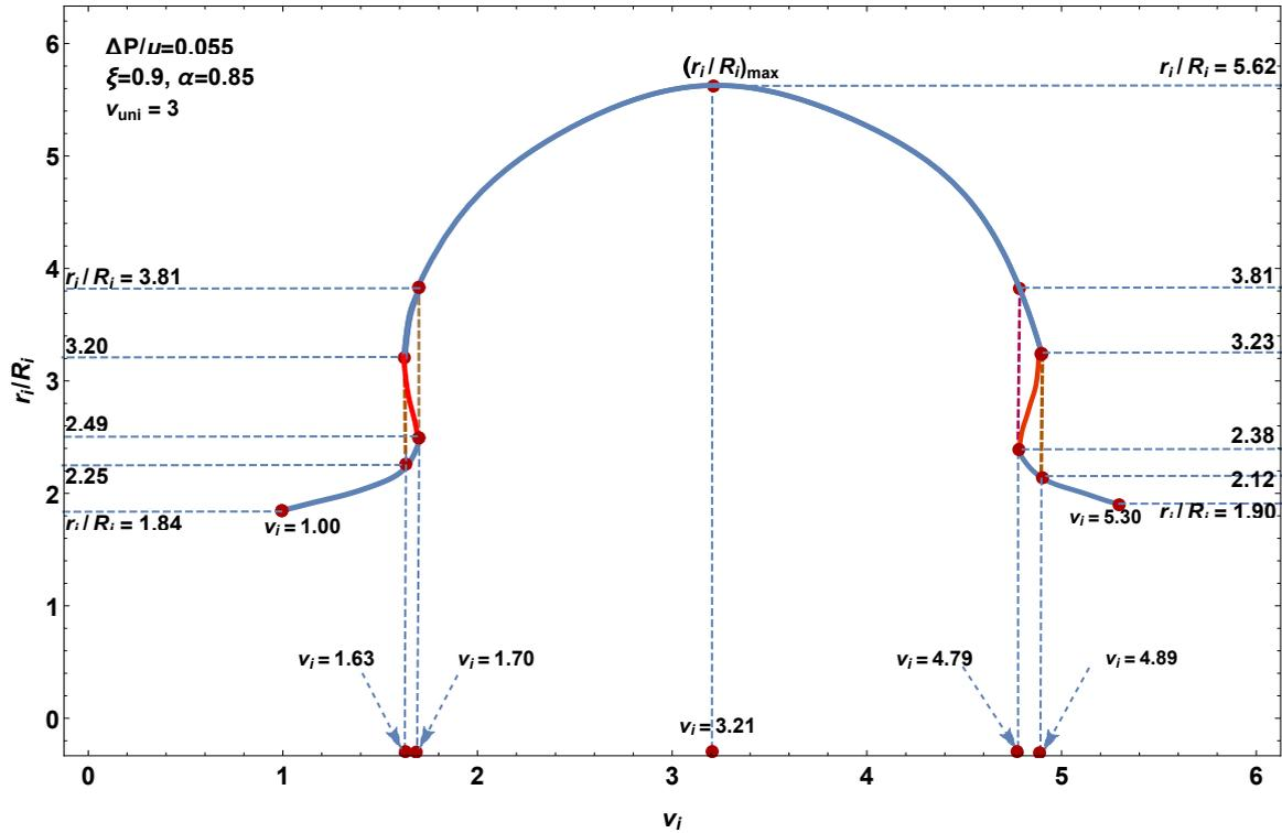
**Figure 12.** Inflation in terms of  $r_i/R_i$  as  $v_i$  varies for (33) with  $\Delta V/R_i^3 = 3.20$ , which again corresponds to the inflation graphs in figures 5 and 6. Here  $\Delta P/\mu = 0.055\mu$ . In contrast to Figure 11, the graph is not a single valued function of  $v_i$ .
