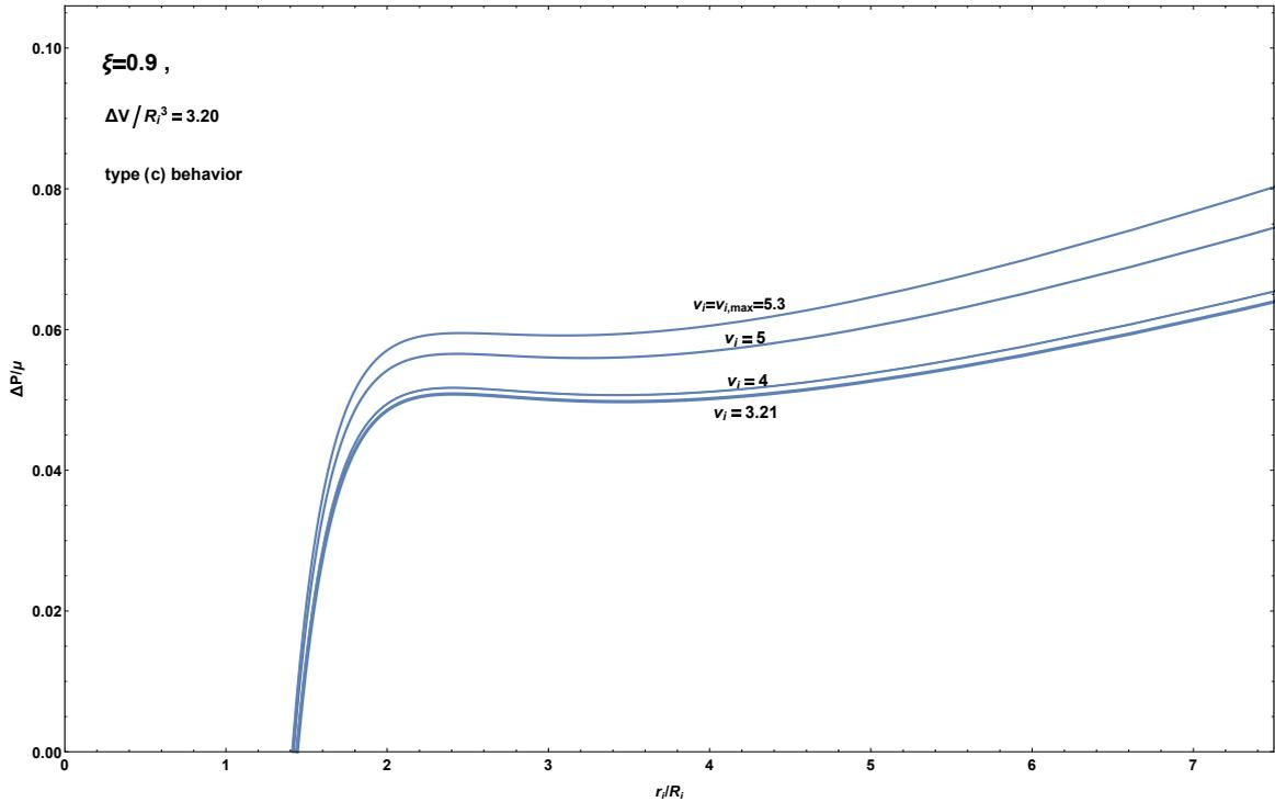
**Figure 6.** Subfamily of inflation graphs for (33) with  $\Delta V/R_i^3 = 3.20$  corresponding to  $3.21 < v_i \leq 5.3 = v_i^{\max}$ . The complete family of inflation graphs  $1 \leq v_i \leq v_i^{\max}$  is accounted for by combining these graphs with those from Figure 5.
