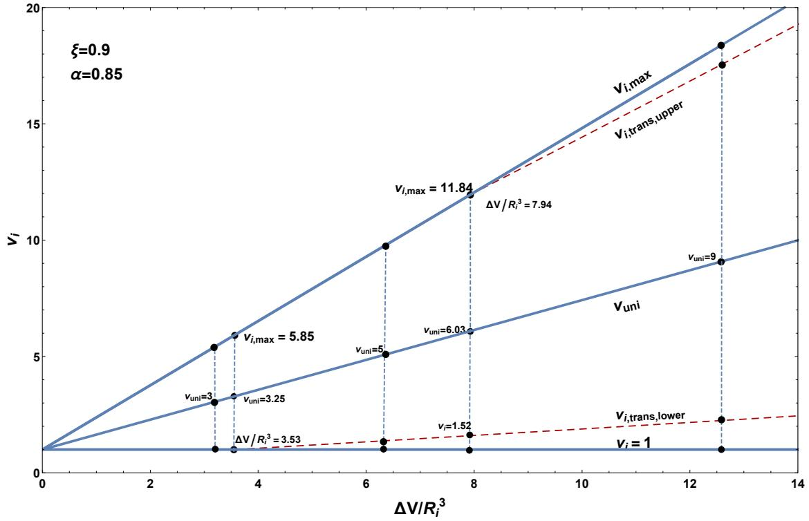
**Figure 4.** The value  $v_i$  on the interval  $1 \leq v_i \leq v_i^{\max}$  parameterizes harmonic swelling fields, all of which have the same added mass content  $\Delta V$ . For a given value of  $\Delta V$  each of these parameterized families correspond to a vertical line segment on this figure, which here is for  $\xi = 0.9$ . The significance of the other curves is developed throughout the text narrative of Section 4.
