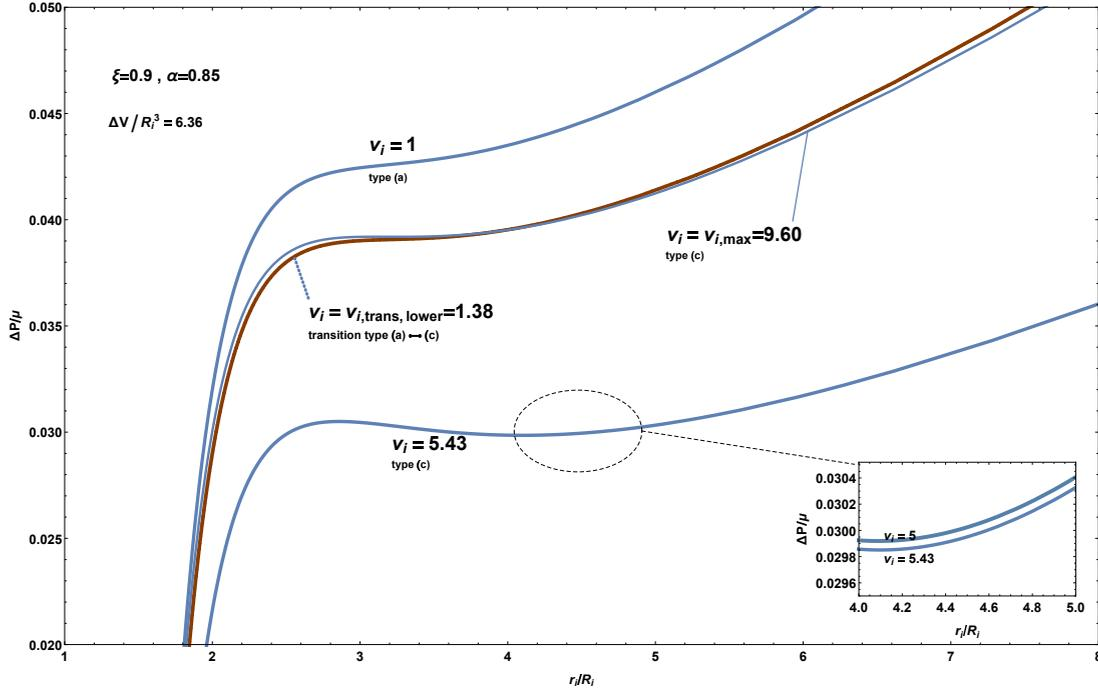
**Figure 7.** The family of inflation graphs for (33) with  $\Delta V/R_i^3 = 6.36$  (which makes  $v_{uni} = 5.0$  and  $v_i^{max} = 9.60$ ). Some remain type-(c) but others are now type-(a). The transition between the two behaviors is the particular inflation graph for  $v_i = v_{i,trans,lower}$  which is shown in red.
