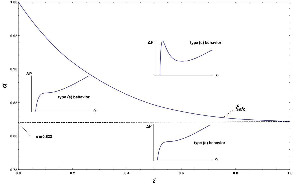
**Figure 2.** Qualitative behavior of the inflation graph for the Mooney–Rivlin model  $W$  given by (5) in the absence of swelling ( $\nu = 1$ ). The curve  $\xi = \xi_{a/c}$  provides a transition between type-(c) and type-(a) behaviors.
