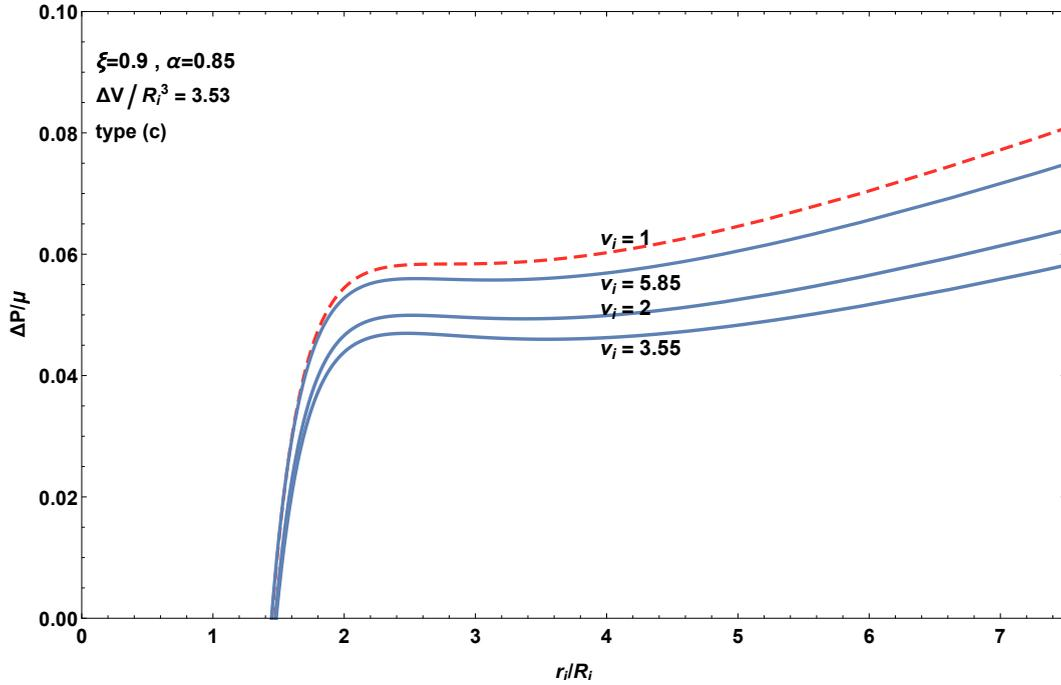
**Figure 8.** The family of inflation graphs for (33) with  $\Delta V/R_i^3 = 3.53$  (which makes  $v_{\text{uni}} = 3.25$  and  $v_i^{\text{max}} = 5.85$ ). The value  $\Delta V/R_i^3 = 3.53$  provides the transition between the family type shown in figures 5 and 6 (always type-(c)) and the family type shown in Figure 7 (sometimes type-(c) and sometimes type-(a)).
