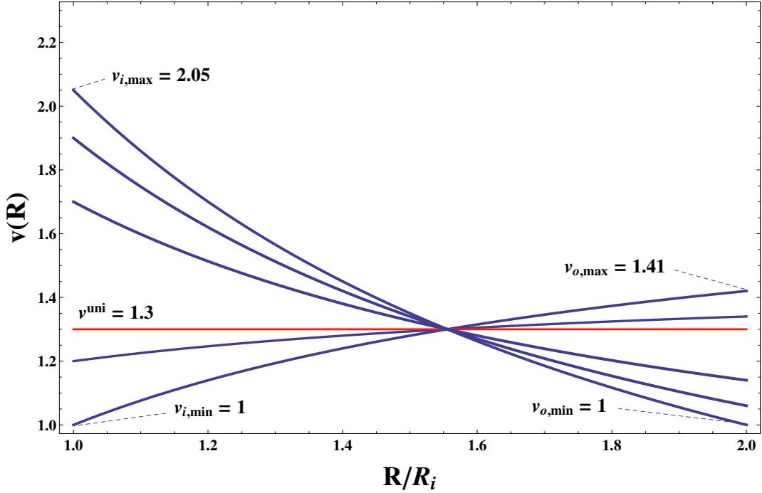
**Figure 3.** The family of harmonic swelling distributions (23) with constants (28) that are parameterized with respect to  $v_i$  such that  $v(R) \geq 1$ . Here  $\xi = 0.5$ . All distributions have the same amount of overall added mass associated with  $v_{\text{uni}} = 1.3$  (30% increase in wall volume from the reference configuration that contains no free liquid).
