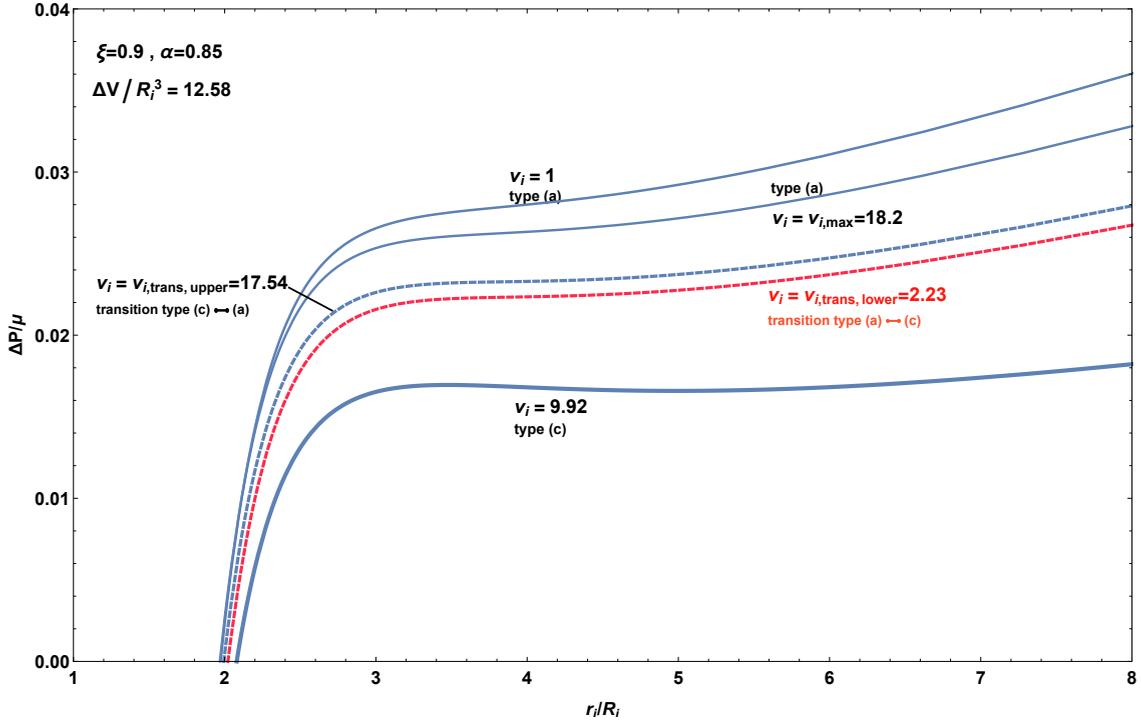
**Figure 9.** The family of inflation graphs for (33) with  $\Delta V/R_i^3 = 12.58$  (which makes  $v_{\text{uni}} = 9.0$  and  $v_i^{\text{max}} = 18.2$ ). Now the behavior is type-(c) for  $v_i$  near  $v_{\text{uni}}$  but type-(a) both near  $v_i = 1$  and near  $v_i = v_i^{\text{max}}$ .
