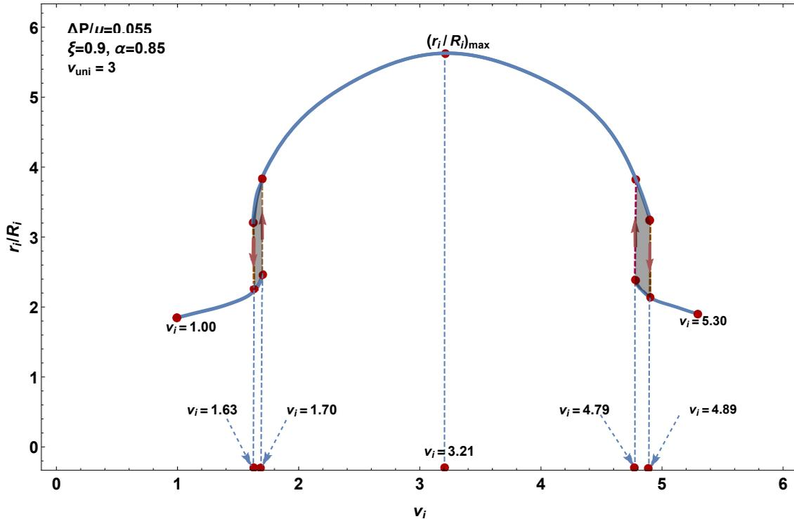
**Figure 13.** Because the graph in Figure 12 does not establish  $r_i$  as a single valued function of  $v_i$ , the swelling agent redistribution involves abrupt jumps (limited bursts of inflation). These are restricted to the transition regions as shown. One possibility is the classical hysteresis behavior that involves jumps at the endpoints of the transition regions (red arrows).
