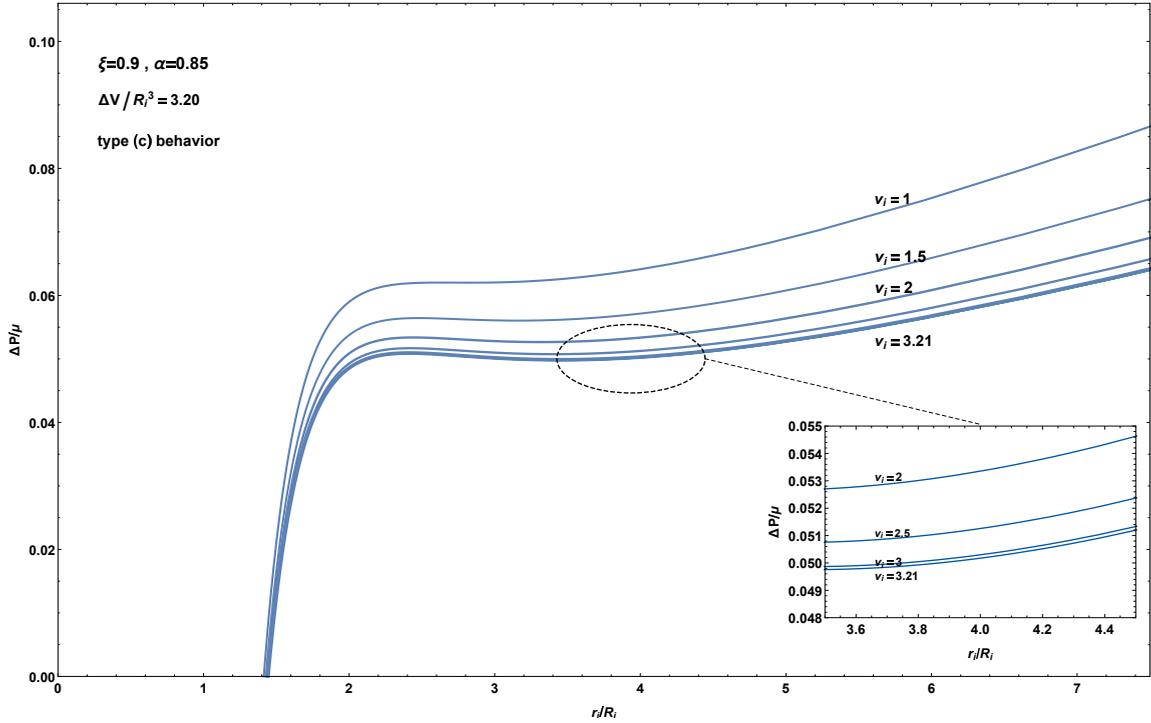
**Figure 5.** Inflation graphs for (33) with  $\Delta V/R_i^3 = 3.20$  (which makes  $v_{\text{uni}} = 3.0$  and  $v_i^{\text{max}} = 5.3$ ). The graphs here correspond to  $1 \leq v_i < 3.21$  which is the subfamily (of the overall family  $1 \leq v_i \leq 5.3$ ) for which the graphs become lower as  $v_i$  increases.
