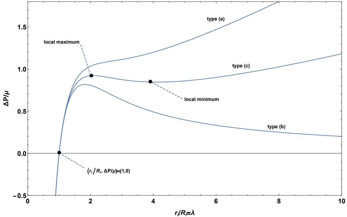
**Figure 1.** Inflation graphs showing three qualitatively different types of behavior (a)-(c) when there is no swelling ( $v = 1$ ). These particular graphs correspond to  $W$  in (5), all with thickness ratio  $R_i/R_o = 0.5$ . The differences are due to the value of  $\alpha$ . Here:  $\alpha = 0.8$  (top curve);  $\alpha = 0.9$  (middle curve); and  $\alpha = 1$  (bottom curve).
