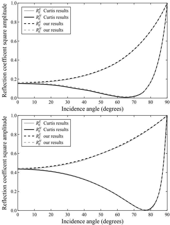
**Figure 4.** Square amplitude of the reflection coefficient for the electric field as a function of the incidence angle in both polarizations. The stratified medium is located below an air half-space and composed of a layer of moist soil 5 cm (top) and 20 cm (bottom) thick on an infinite layer of dry soil.
