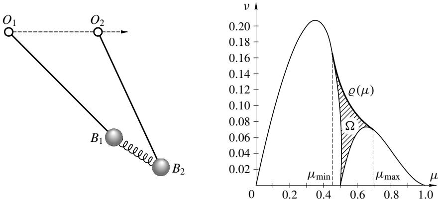
**Figure 4.** Left: the asymmetric classical configuration in the region A1. Right: the stability domain  $\Omega$  of the asymmetric classical configuration in the region A1.
