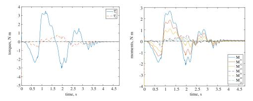
**Figure 8.** Closed loop trajectory: joint torques (left), and lumped moments (right).
