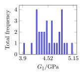
**Figure 10.** Experimental results and identification for fiber orientation 45°: (left) maximal shear stress  $\sigma_{12}$  versus maximal shear strain  $\gamma_{12}$  curves and (right) frequency distribution of shear modulus in fiber direction  $G_{\parallel}$ .
