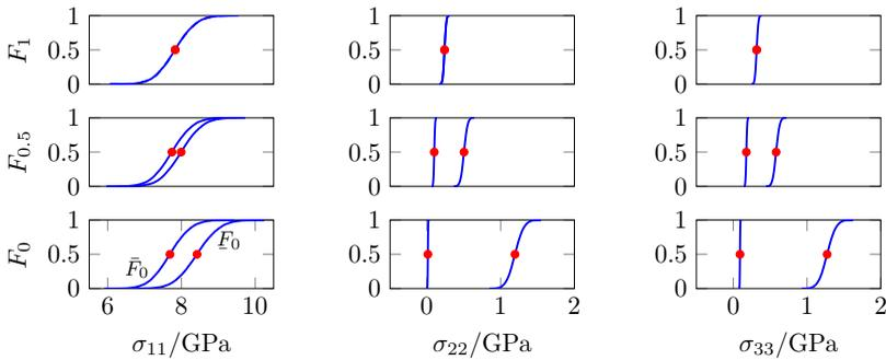
**Figure 16.** Fuzzy-stochastic analysis: P-boxes at  $\alpha$ -levels  $\alpha_1 = 0$ ,  $\alpha_6 = 0.5$  and  $\alpha_{11} = 1$  for normal stresses (left)  $\sigma_{11}$ , (center)  $\sigma_{22}$ , and (right)  $\sigma_{33}$ .
