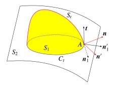
**Figure 1.** A drop lies on solid surface  $\mathcal{G} = S_1 \cup S_2$ ;  $S_t$  is a free surface;  $n_1$  and n are the external unit normal vectors to  $S_1$  and  $S_t$ , respectively. Contact line  $C_t$  separates  $S_1$  and  $S_2$ , t is the unit tangent vector to  $C_t$  on  $\mathcal{G}$ . Vectors  $n'_1 = n_1 \times t$  and  $n' = t \times n$  are the binormals to  $C_t$  relative to  $\mathcal{G}$  and  $S_t$  at point A of  $C_t$ , respectively.
