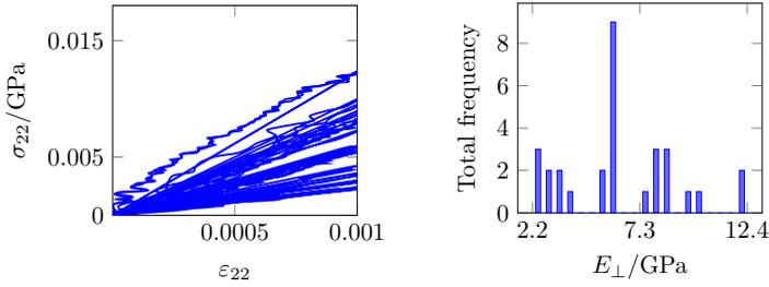
**Figure 9.** Experimental results and identification for fiber orientation  $90^\circ$ : (left) curves for stress  $\sigma_{22}$  transversal to fiber versus strain  $\epsilon_{22}$  transversal to fiber and (right) frequency distribution of Young’s modulus in transverse direction  $E_{\perp}$ .
