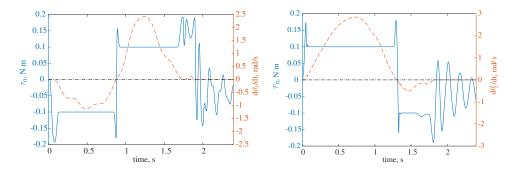
**Figure 5.** Straight trajectory: friction torque  $\tau_{\mathfrak{f}1}$  and  $\dot{\vartheta}_1$  (left), and friction torque  $\tau_{\mathfrak{f}2}$  and  $\dot{\vartheta}_2$  (right).
