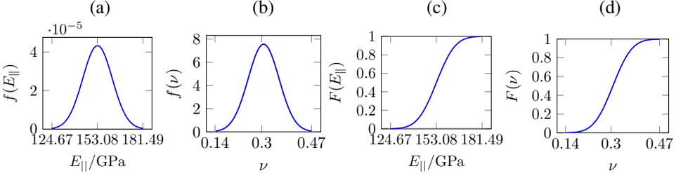
**Figure 14.** Fuzzy-stochastic analysis: input density functions for the aleatory material parameters (a) PDF for  $E_{\parallel}$ , (b) PDF for  $\nu$ , (c) CDF for  $E_{\parallel}$ , and (d) CDF for  $\nu$ .
