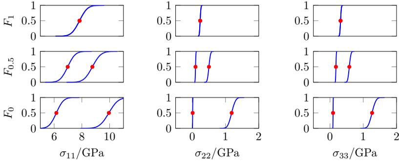
**Figure 22.** Hybrid fuzzy-stochastic analysis: P-boxes at  $\alpha$ -levels  $\alpha_1 = 0$ ,  $\alpha_6 = 0.5$  and  $\alpha_{11} = 1$  for normal stresses  $\sigma_{11}$ ,  $\sigma_{22}$ ,  $\sigma_{33}$ .
