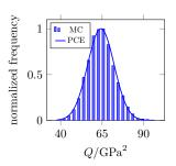
**Figure 2.** PCE and MC distribution of Young's modulus  $E(\omega)$  (left) and QoI  $Q(\omega)$  (right) of (24) and (27), respectively.
