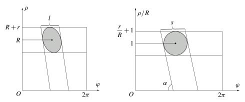
**Figure 5.** The control area of one circle of radar scan in the polar coordinate system (left) and in the normalized polar coordinate (right) associated with moving vehicles.
