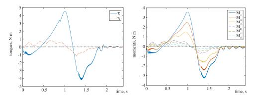
**Figure 4.** Straight trajectory: joint torques (left), and lumped moments applied to  $\varphi_{ij}$  (right).
