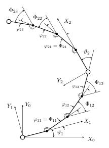
**Figure 1.** Discrete system corresponding to a planar two-link flexible arm.
