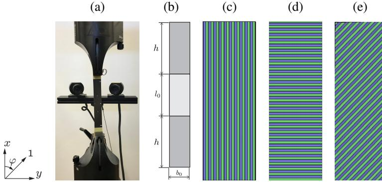
**Figure 6.** Experimental investigation: (a) experimental setup, (b) geometry of specimens, and schematic specimens for fiber orientation (c)  $0^\circ$ , (d)  $90^\circ$ , and (e)  $45^\circ$ . Machine-fixed coordinate system  $(x, y)$  and fibers aligned to 1-axis.
