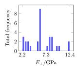
**Figure 9.** Experimental results and identification for fiber orientation 90°: (left) curves for stress  $\sigma_{22}$  transversal to fiber versus strain  $\varepsilon_{22}$  transversal to fiber and (right) frequency distribution of Young's modulus in transverse direction  $E_{\perp}$ .
