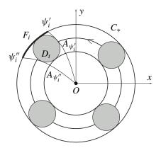
**Figure 4.** Control area of one circle of radar scan in the Cartesian coordinate system (x, y) associated with moving vehicles.
