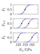
**Figure 19.** Hybrid fuzzy-stochastic analysis: P-boxes at  $\alpha$ -levels  $\alpha_1 = 0$ ,  $\alpha_6 = 0.5$ , and  $\alpha_{11} = 1$  for  $E_{\parallel}$ .
