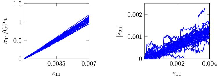
**Figure 7.** Experimental results for fiber orientation  $0^\circ$ : (left) longitudinal stress  $\sigma_{11}$  versus longitudinal strain  $\epsilon_{11}$  curves and (right) longitudinal strain  $\epsilon_{11}$  versus transversal absolute strain  $|\epsilon_{22}|$  curves.
