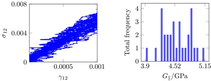
**Figure 10.** Experimental results and identification for fiber orientation  $45^\circ$ : (left) maximal shear stress  $\sigma_{12}$  versus maximal shear strain  $\gamma_{12}$  curves and (right) frequency distribution of shear modulus in fiber direction  $G_{\parallel}$ .
