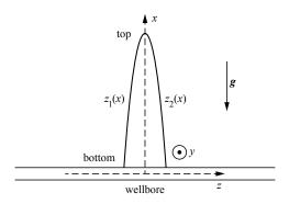
**Figure 1.** Schematic representation of the fracture.
