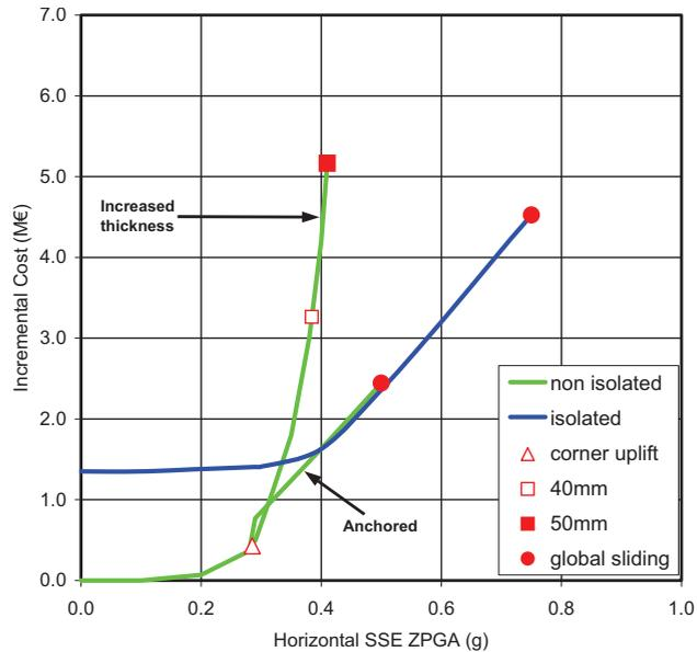
**Figure 6.** Cost evolution with seismic demand: pile foundation.
