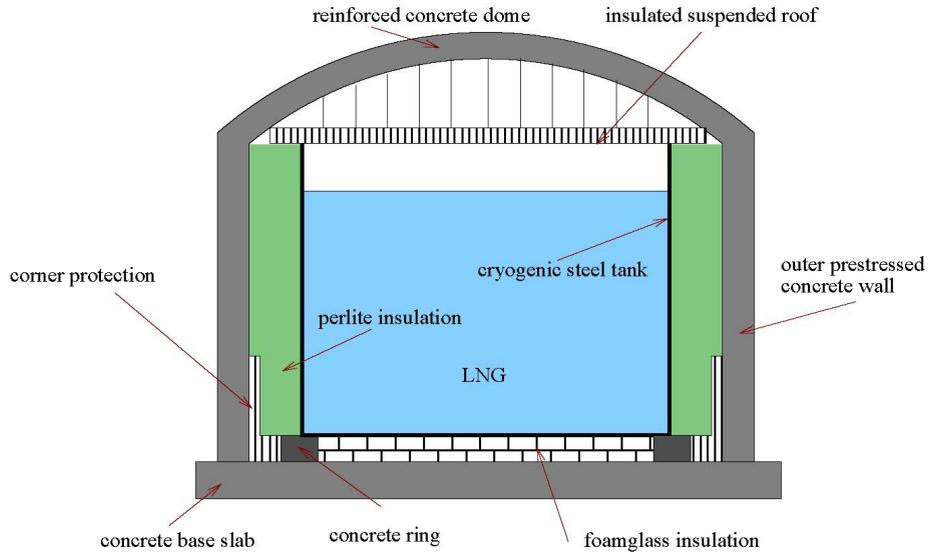
**Figure 1.** Schematic view of a modern LNG tank.
