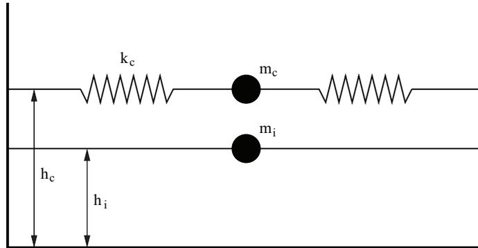
**Figure 3.** Effective liquid masses in horizontal oscillations.
