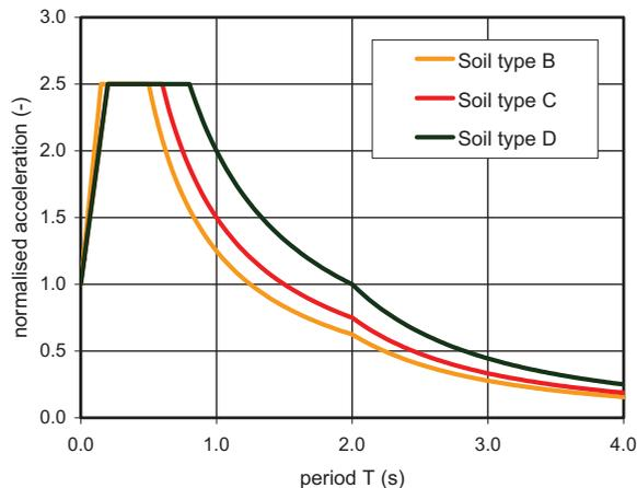
**Figure 2.** Spectral shapes used in the calculations.
