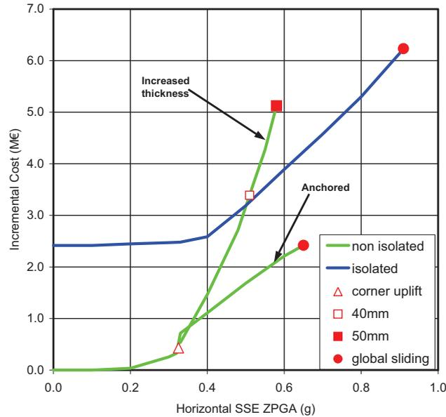
**Figure 5.** Cost evolution with seismic demand: slab foundation.
