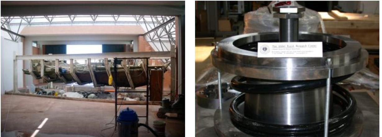
**Figure 47.** The wooden Roman ship excavated at Herculaneum, near Naples, in seismic zone 2, which was recently protected in the local museum by means of 3D isolators formed by three spheres and a re-centering rubber cylinder for the horizontal SI and a spring and a VD for the vertical one.
