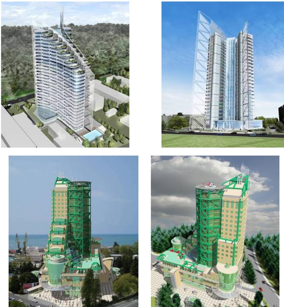
**Figure 17.** Top: new Sea Plaza Hotel at Sochi (27 storeys, in addition to 2 underground ones; height  $\approx 93$  m; total living area =  $40,000$  m<sup>2</sup>), protected by 102 HDRBs. Bottom: new r.c. commercial center, with cinema, underground parking and offices, again at Sochi (21 storeys, in addition to the ground and 2 underground floors; height  $\approx 100$  m; total living area =  $50,000$  m<sup>2</sup>), protected by 200 LRBs.
