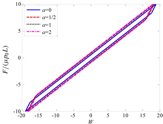
**Figure 8.** Effect of pressure distribution laws on the hysteresis loop.
