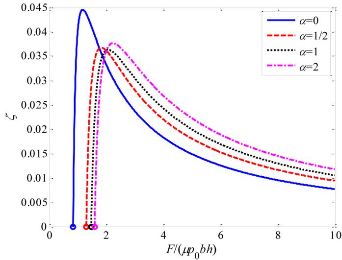
**Figure 10.** Plots of the relationship between damping ratio and nondimensional normal load for different pressure distribution laws. The symbol  $\circ$  denotes the minimum force values inducing relative slip.
