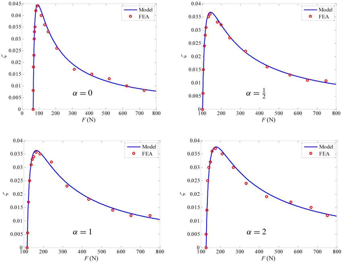
**Figure 17.** Comparison of damping ratio versus normal load between model predictions and FEA results for different pressure distribution laws.
