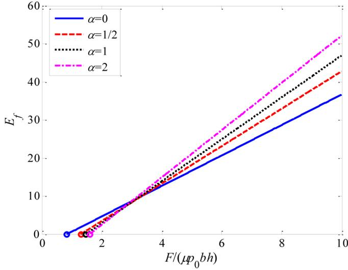
**Figure 6.** Nondimensional energy dissipation as a function of nondimensional normal load for different pressure distribution laws. The symbols  $\circ$  is for the minimum force values inducing relative slip.
