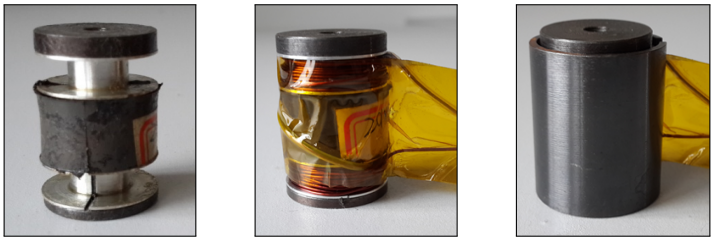
Figure 6. Different assembly forms of MRE isolator: compound structure (left), compound structure with coils (middle), and complete structure (right).
