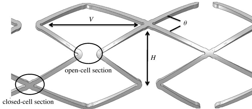
**Figure 3.** Representation of the stent cell specifications of the stents used in this work ( $V$  stands for the distance in axial direction,  $H$  the distance in circumferential direction and  $\theta$  the inter-strut angle).
