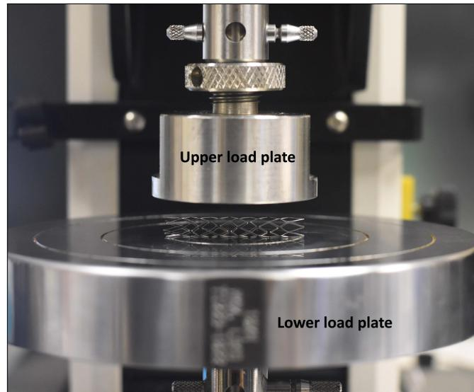
**Figure 6.** Experimental setup for radial compression test.
