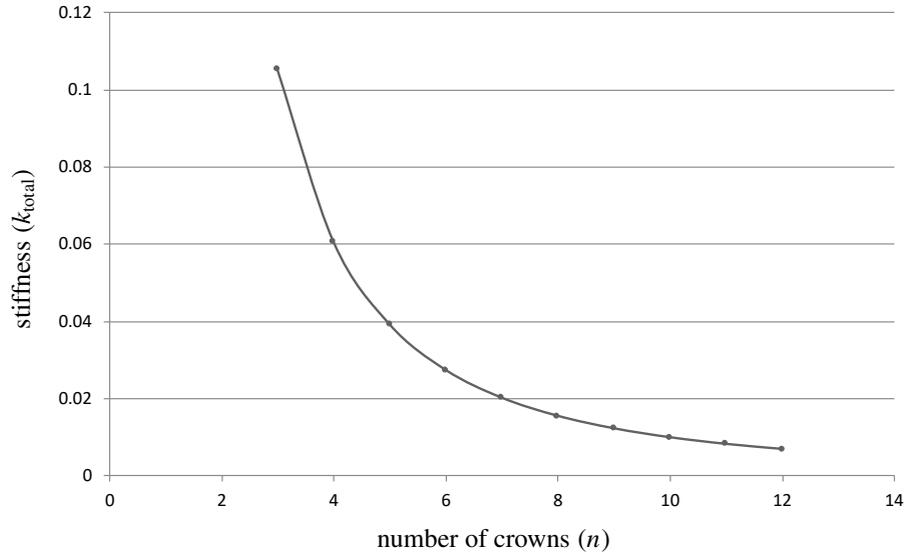
**Figure 10.** Total stiffness vs number of crowns with the value of  $k_{total}$  as a function of  $n$  according to (3).
